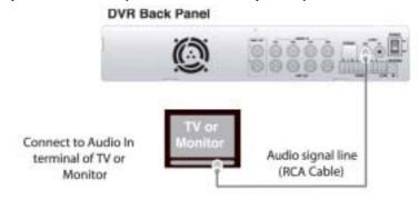
Using an RCA cable, connect the AUDIO IN terminal of your TV / monitor to the AUDIO OUT terminal of your DVR rear panel.
